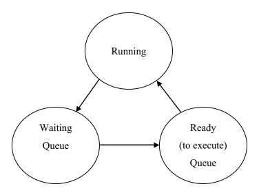
Figure 7-1 RTOS Task states diagram
